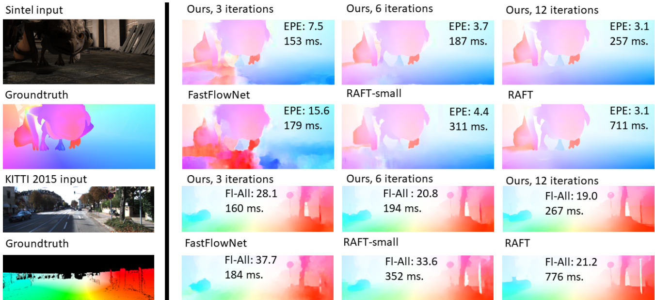
Fig. 5. Qualitative results of comparable methods at different time requirements. Our method can be as fast as FastFlowNet while producing noticeably better results. We can also increase the number of refinements and achieve results comparable to RAFT while running at almost three times its speed.
