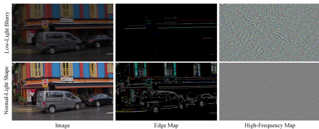
Fig. 2. A visual comparison of edge and high-frequency maps of the low-light blurry image, and normal-light sharp image.
