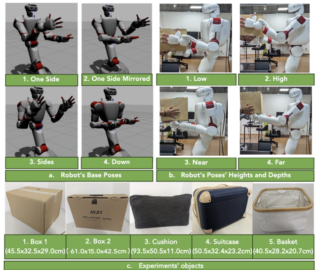
Fig. 2. Experiment setting overview. From left to right – a. Robot’s base poses. Poses vary in x and y coordinates based on the handed-over object, height, and depth variations. b. Robot’s poses’ heights and depths c. Experiments’ objects and corresponding sizes (width × depth × height).
