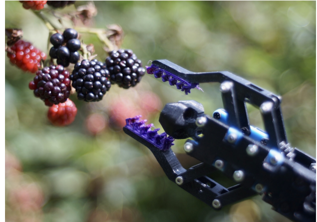
Fig. 1: Compliant gripper in situ in a blackberry farm, shown without integrated ripeness sensor for clarity. The three-berry cluster in foreground contains representative ripe (right-most two) and near-ripe (on the left) blackberries.
