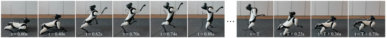
Fig. 3: Our RL policy brings up the quadrupedal robot from a lying pose to a stabilized bipedal standing pose. The separate sit-down policy then controls the robot from the upright standing pose to settle down with four legs on the ground. The learned policies demonstrate great agility, using less than 1 second to stand up and sit down, while are sufficiently robust to work on the real robot.
