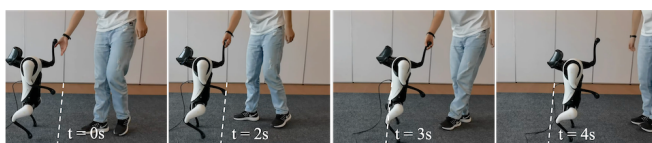
Fig. 9: A human walks hand-in-hand with the standing quadruped robot and drags its front leg to change its position.
