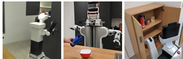
Fig. 9. Photos from the auxiliary experiments with different robots performing mobile manipulation actions. (left) One-shot detections for pick & place and pouring actions. (middle) A continuous perception task with object tracking. (right) HSR in a RoboCup@Home scenario. Details are available at https://robokudo.ai.uni-bremen.de/rkop .
