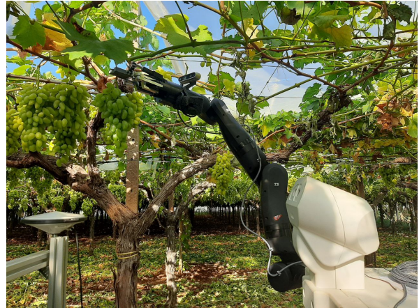
Fig. 1: Agricultural robotic platform used in the EU Project CANOPIES for operations in table grape vineyards, equipped with an Intel RealSense d435i camera on the wrist. AgriSORT is implemented on this robot, and is used for tracking grapes.
