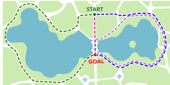
Fig. 1: The robot navigates from one side of the lake to the other. If the bridge is likely to be traversable, the roadmap should include the pink path so that the robot can inspect the bridge’s traversability, as well as the two purple paths to allow the robot to go across the bridge if it is traversable and around the lake if it is not. If the bridge is likely untraversable, including those paths in the roadmap only increases planning complexity without significantly improving planning performance. A sparser graph that only has the blue path would still result in plans with expected near-optimal costs. Since the green and blue paths are both known to be traversable, including the longer green path in the roadmap is never useful.
