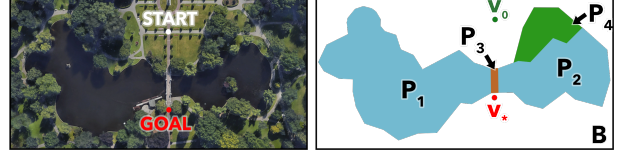
Fig. 2: The robot is tasked with navigating through a park. The bridge over the lake may or may not be traversable. We abstract the key regions in the environment as polygons (using e.g., a semantically segmented overhead image): P_1 and P_2 represent the lake, which is known to be untraversable. P_3 represents the bridge, which has a 50% chance of being traversable. P_4 represents the grove of trees, which has a 30% chance of being traversable. In the weather w = \{0, 0, 1, 1\} , the bridge and forest are traversable, while the lake is untraversable.
