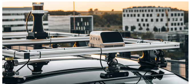
Fig. 3. Sensor rack of research vehicle; as the rest of the software stack, the drivers for the sensors are each running in their own minimal container.
