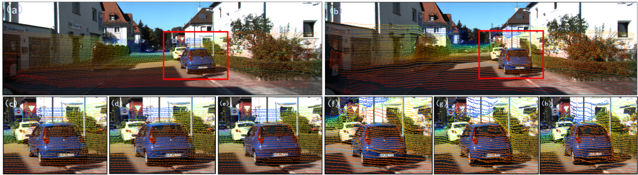
Fig. 5: We show the qualitative results of HIFMNet and its calibration flow revision HIFMNet(flow). (a)(b) are calibration and flow estimation results of HIFMNet and HIFMNet(flow) after first extrinsic update iteration. We enlarge the areas within the red boxes. (c)(d)(e) and (f)(g)(h) are results after first, second and fourth iterations. Even with an increase in the iteration number of HIFMNet(flow), noticeable distortion patterns still exist.
