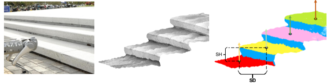
Fig. 1: Staircase environment, staircase detection and modeling. The image illustrates the traversable regions predicted by our framework, with arrows indicating estimated normals. Ellipses positioned beneath the arrows represent center point estimations. The abbreviation 'SH' means step height, while the 'SD' refers to the step depth. The raw output of modeling is refined through measurement correction to derive stair parameters. Our method demonstrates robustness and accuracy across diverse lighting conditions and viewpoints, offering a reliable solution for robotic stair navigation in real-time.
