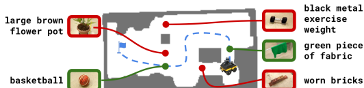
Fig. 4: The Jackal robot solving a traversability challenge. All paths to the goal are obstructed by objects. We query an LLM to identify which objects can be safely pushed or traversed by the robot (green) and which objects would be too heavy or hinder the robot’s movement (red). The LLM relies on the ConceptGraphs node captions to make traversability predictions and we add the non-traversable objects to the Jackal costmap for path planning. The Jackal successfully reaches the goal by going through a curtain and pushing a basketball, while also avoiding contact with bricks, an iron dumbbell, and a flower pot.
