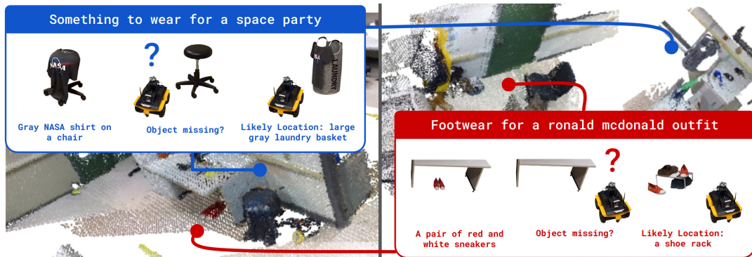
Fig. 3: A Jackal robot answering user queries using the ConceptGraphs representation of a lab environment. We first query an LLM to identify the most relevant object given the user query, then validate with an LVLM if the target object is at the expected location. If not, we query the LLM again to find a likely location or container for the missing object. (Blue) When prompted with something to wear for a space party, the Jackal attempts to find a grey shirt with a NASA logo. After failing to detect the shirt at the expected location, the LLM reasons that it could likely be in the laundry bag. (Red) The Jackal searches for red and white sneakers after receiving the user query footwear for a Ronald McDonald outfit. The LLM redirects the robot to a shoe rack after failing to detect the sneakers where they initially appeared on the map.
