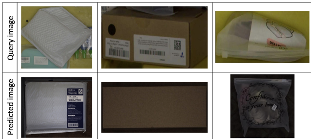
Fig. 8. Failure cases: (Top) the query image, (Bottom) highest confidence match. In all these cases, the correct item only had catalog image as reference source which was not representative of the appearance.
