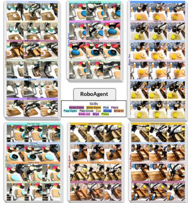
Fig. 1: A glimpse of the diverse manipulation capabilities of RoboAgent — a single agent capable of 12 manipulation skills across 38 tasks encompassing 6 activities. For videos, visit: https://robopen.github.io
