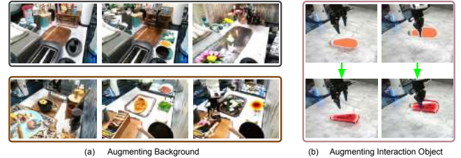
Fig. 5: Illustration of the data augmentations used to rapidly multiply limited robot datasets with diverse semantic scene variations. (a) shows the scene around the robot and the interaction object changing. (b) shows the interaction object itself changing while preserving the rest of the scene.
