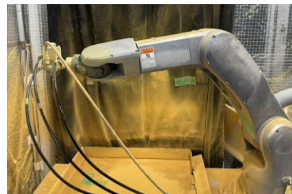
Fig. 1. This picture shows the painting robot used in this study. The painting robot has a painting gun attached at the end of its robot arm.
