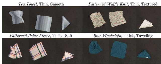
Fig. 8. Our method can generalize to fabrics of a variety of appearances and textures. We show the initial, smooth state before folding, and final configurations from successful folding episodes.
