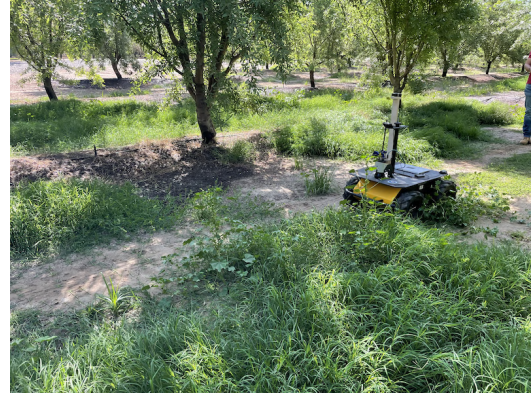
Fig. 1: A robot navigating in an almond orchard facing high weeds and bushes that are classified as obstacles by the standard ROS 2 navigation stack, but that can be safely traversed.
