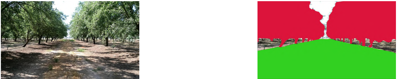
Fig. 6: Example of ground truth manual annotation in the dataset: (a) Original image and (b) Image with manually applied labels. Red pixels correspond to “obstacle”, while green pixels correspond to “traversable”.
