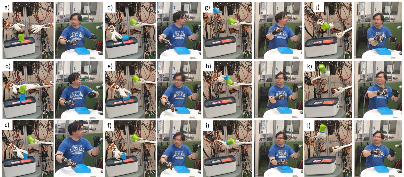
Fig. 7: Bimanual manipulation task of stacking cups. Subfigure a) and b) show the green cup being picked up by the left hand. Subfigures c), d), and e) show the right hand re-orienting the blue cup to an upright position for grasping, as shown in Subfigure f). Subfigure g) and h) show the blue cup being inserted into the green cup and Subfigures i), j), k), and l) show the stacked cups being transferred to the right hand and reoriented on the right hand.
