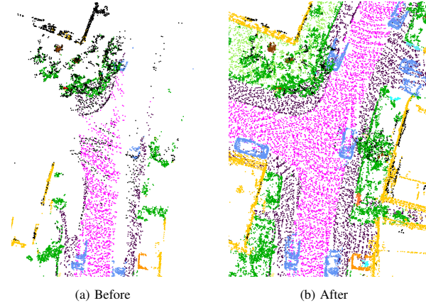
Fig. 1. An example of our adaptive voxel map. (a) and (b) show how our local map is updated before and after the mobile robot passes through the intersection. Points without semantic information (marked in black) are gradually replaced with semantic points.
