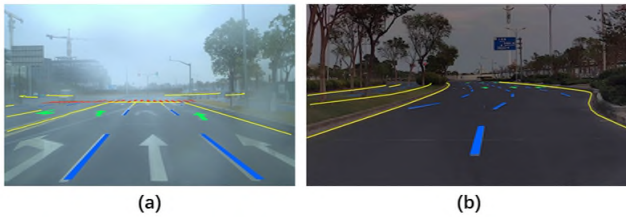
Fig. 8. (a) is the projection of the map on the image without z-axis correction, and the lane line projection of the map and the lane lines in the image are not aligned. (b) is the projection of the map on the image with z-axis correction.
