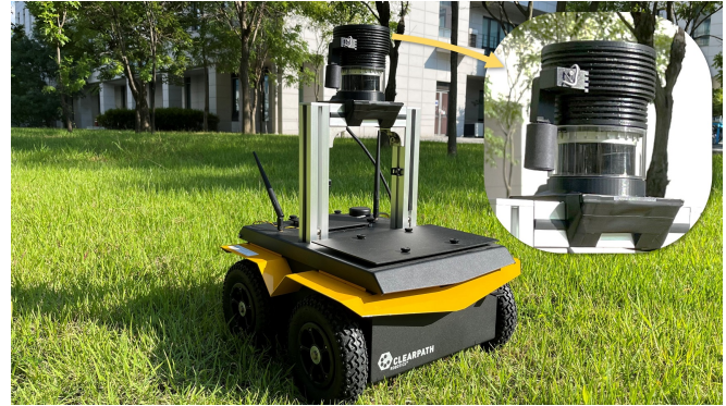
Fig. 1. LiDAR protection module for outdoor unmanned vehicles.
