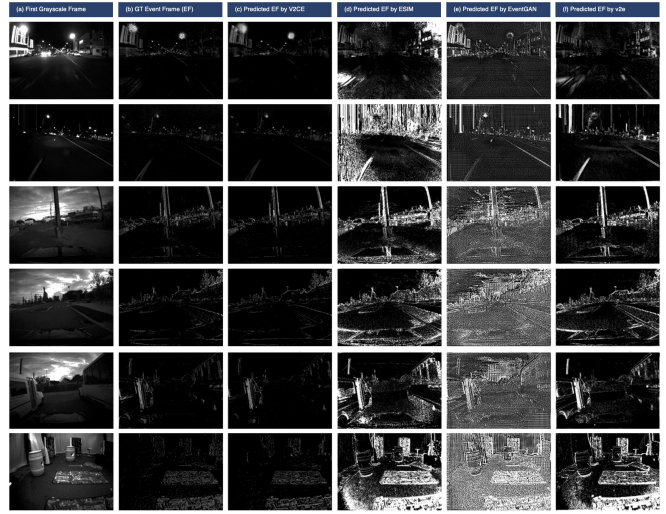
Fig. 4. Event frame comparison between V2CE and baseline methods. Event frames are clipped to the maximum value of their corresponding ground truth event frames and then normalized.
