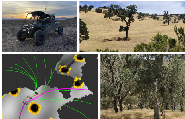
Fig. 1: Clockwise from the top left: The Polaris RZR vehicle used for data collection; two example environments showing hilly and forested areas, respectively; visualization of the risk-predictive planner in action, showing the selected trajectory (magenta) alongside rejected candidate paths (green) overlaid on an elevation-mapped occupancy map with unknown regions due to terrain occlusions.
