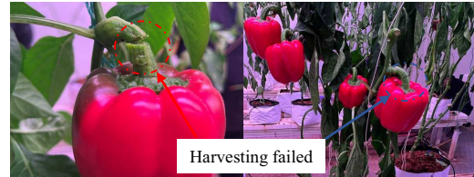
Fig. 15. A case of failure in harvesting sweet peppers.
