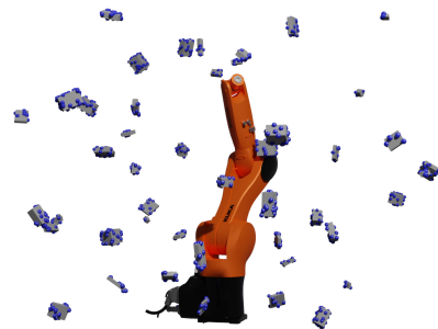
Fig. 5: An example of a box world scene, with randomly sampled boxes and points on the surface of the boxes.
