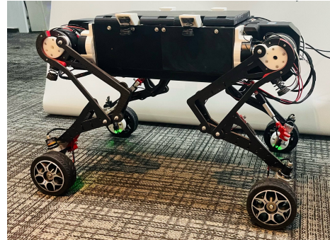
Fig. 1: Pegasus: the bio-inspired wheeled-quadruped robot.
