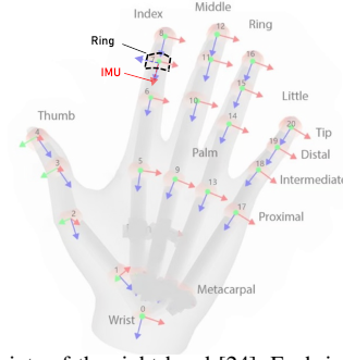
Fig. 3. The 21 joints of the right hand [24]. Each joint has a number ID.
