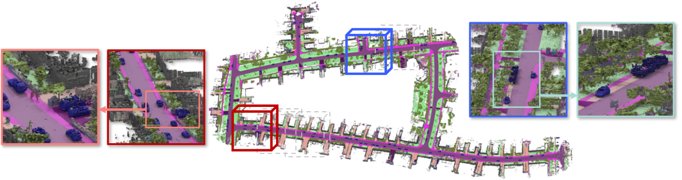
Fig. 2. The center image shows the semantic reconstruction of the global map using LiDAR and semantic labels on Seq.00 of the KITTI-360. Several example volumes are shown in the map, among which the red and blue ones are highlighted with the surface details in the side images.
