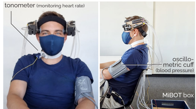
Fig. 6. The experimental setup during MiBOT's evaluation included a tonometer on the carotid artery to measure heart rate as well as an oscillometric cuff to take blood pressure measurements.
