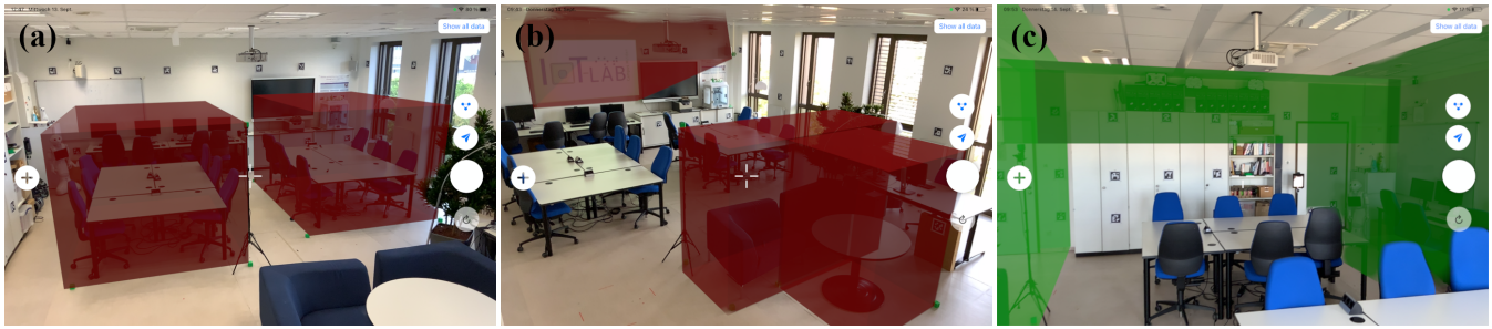
Fig. 4. Three use cases for more complex scenarios of virtual borders. Image (a) and (b) show a combination of multiple cuboid areas the robot should avoid. Image (c) shows two defined working areas connected by a flight corridor the robot should not leave. Area boundaries are again defined by real green cubes. Furthermore, a projector image is used as reference.
