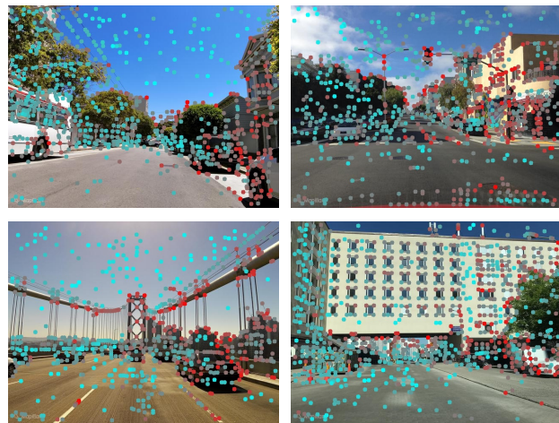
Fig. 3. Visualization of the attention weights computed by SuperGF on the input local features. Red dots indicate local features with high weights and cyan dots indicate those with low weights.
