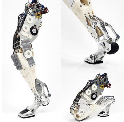
Fig. 1. Developed high-DOF leg and toe mechanism HyperLeg.
