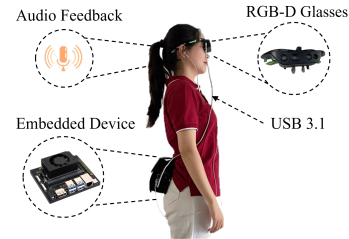
Fig. 1. The hardware of wearable steering assistance. The assistance consists of a pair of RGB-D glasses, an embedded device, and headphones for audio feedback.
