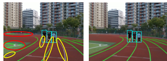
Fig. 5. The valuation result trained on different dataset. The yellow ellipses are the false negative and the red ellipses indicate the false positive.
