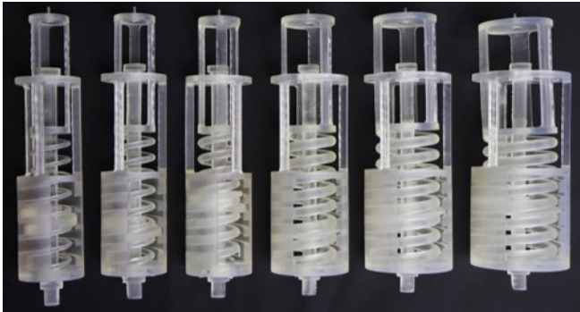
Fig. 6. From left to right: VSMs in configurations 1 to 6 (Table I) after supports removal, IPA cleaning and additional curing in UV chamber.
