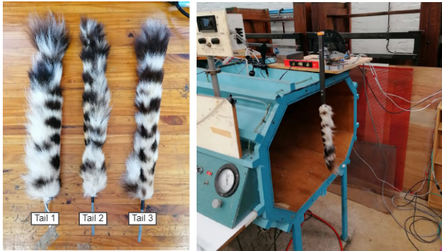
Fig. 3: (Left) The three cheetah tails studied. (Right) A cheetah tail in the wind tunnel.
