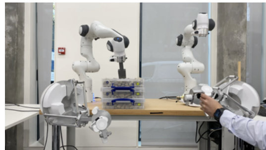
Fig. 1. (a) Haptic : The master moves the replica (Panda, Franka Emika AG) by applying a virtual force ( f_v ). The interaction force/torque feedback at the end-effector ( F_{FB} ) is scaled in A_M to generate the haptic feedback. The operator can also act on the replica end-effector’s reference pose ( x_d ) by activating the master device with its grasp joint or via the GUI. Non-Haptic : The replica is controlled by issuing sequences of x_d that act as via points for the trajectory of the replica. (b) Dual-arm Tele-cooperation Setup.
