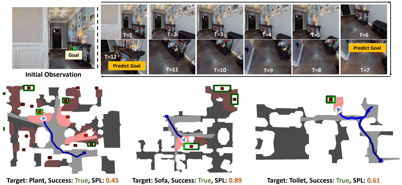
Fig. 5. Trajectory visualization of both PixNav policy and long-horizon object navigation. The top part represents the first-person view of PixNav trajectory. Even though the robot’s view changes constantly, our model can still predict the original goal and walk towards it. The bottom part represents the top-down view of the entire trajectory. Our LLM-based planner helps the robot achieve consistent and semantic exploration towards the target.
