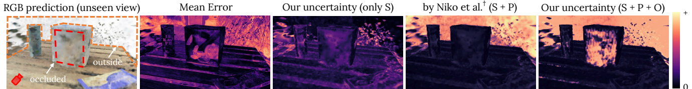
(b) Example of our inferred 2D pixel-wise uncertainty. For the rendered RGB prediction from an unseen view with occlusion and outside scene content, our method is the only one that can correctly estimate uncertainty on all Surface (S), Outside (P) and Occluded (O) points.
