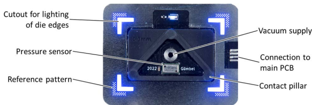
Figure 4. Die-gripper-interface, aluminium PCB and reference pattern with active background illumination.
