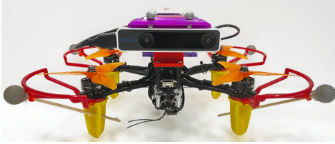
Fig. 7. Platform used for the real-world experiments equipped with a Jetson Xavier computer, an Intel Realsense T265 tracking camera, a PixRacer flight controller, and infrared-reflective markers for motion capture.
