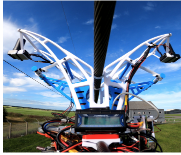
Fig. 5: Gripper engaged by powerline.
