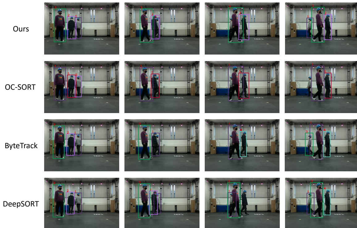
Fig. 4: Example results of LF25 dataset. The flow of time goes from left to right. Whereas current algorithms struggle with lost tracks or ID switching during occlusions, FocoTrack effectively assigns IDs even when three individuals are closely clustered in the occlusion scenario.
