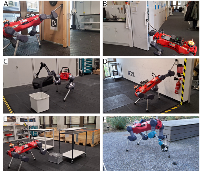
Fig. 1: Our foot target tracking controller enables a variety of real-world manipulation tasks such as opening doors (A) and fridges (B), object transport (C), pressing a button (D), pushing obstacles out of the way (E), and collecting rock samples (F).
