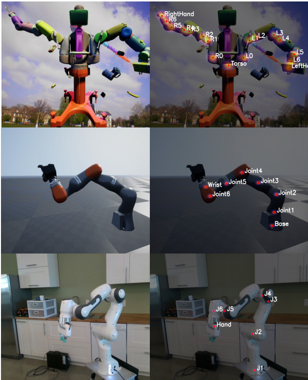
Fig. 4. Belief maps (right column) overlaid on the original images(left column) for Rethink Baxter, Kuka LBR iiwa, Franka Emika Panda from up to down.
