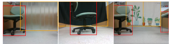
Fig. 3. Examples of output of the large model module. The initial instruction for these examples is: “Please go through the curtain and be careful of the chair”. We obtain the landmarks and the corresponding traversable attributes, curtain and 1 (in orange); chair and 0 (in red), using GPT-3.5. Then, we can ground the related bounding boxes with [23].
