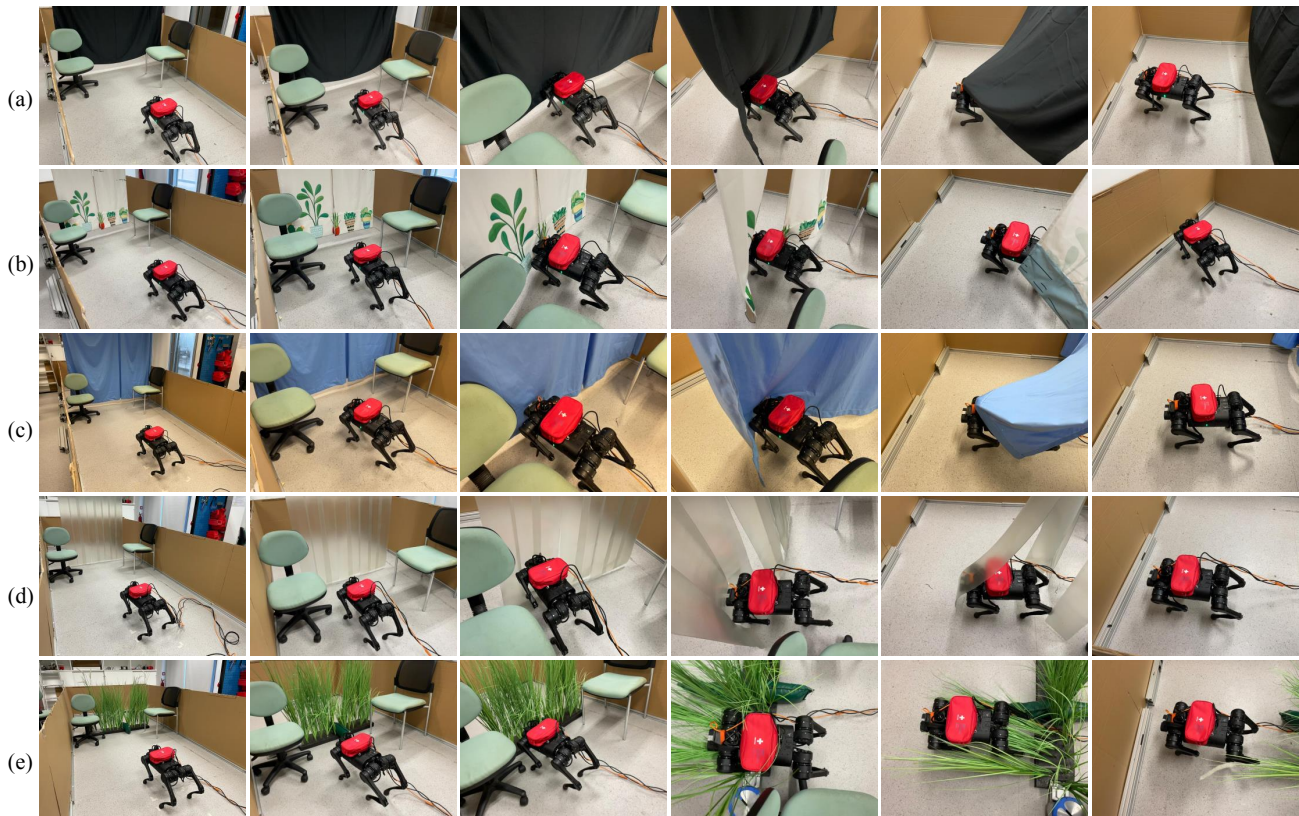
Fig. 7. (a-d) Experiments of going through different curtains. (e) Experiment of going through the grass.
