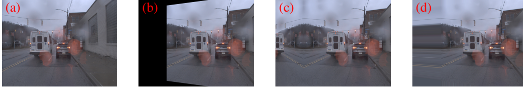
Fig. 5. Different border modes. (a)Original FV image. Augmented FV image with (b)zero border, (c)reflect border, and (d)replicate border.
