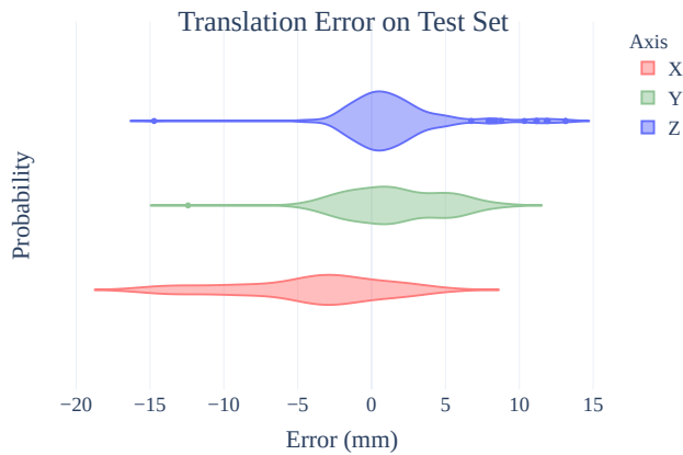
Fig. 8. Translation Error Plot. The data is from 199 samples and only one prediction result is removed due to a wrong bounding box detection. For a better visualization, on this plot the raw values are plotted instead of the absolute error values which are discussed in Sec. V
