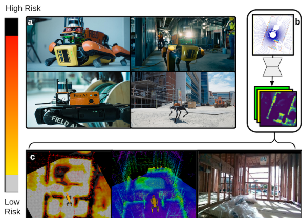
Fig. 1: We propose UNRealNet (b), a network that produces high-quality, robot-agnostic navigation features and traversability (c) directly from pointclouds from an on-board sensor (a). Colormap for risk maps included for clarity.
