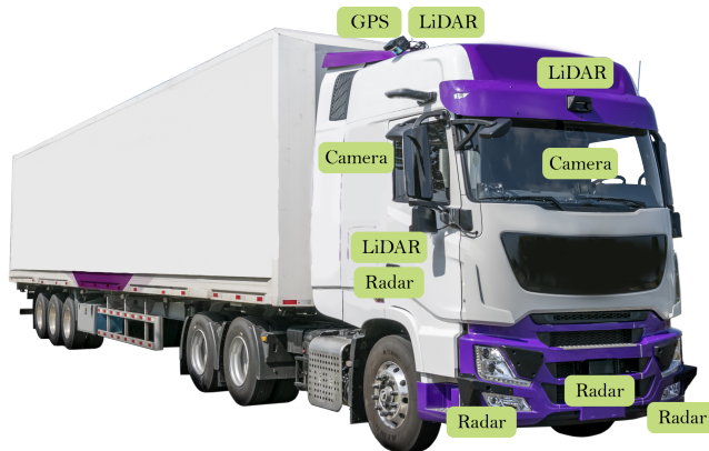
Fig. 2: Sensor setup for the ESP data collection platform involves the Inceptio autonomous truck, which is equipped with 5 LiDARs, 7 cameras, 7 radars, and GPS.
