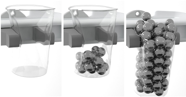
Fig. 4: Simulation of a Franka Emika Hand grasping a plastic cup with weights. Results visualized with Blender’s Cycles path tracer.
